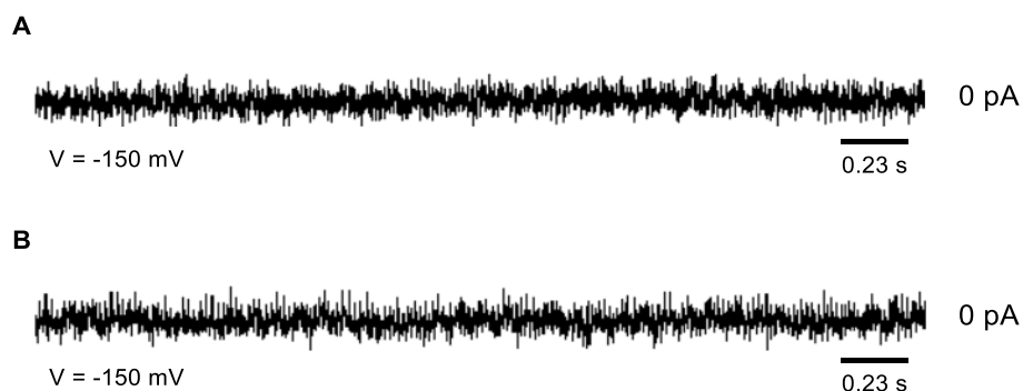
Figure 36: Current traces at the applied voltage of -150 mV under symmetrical KCl (1.0 M) conditions across the diphytanoylphosphatidylcholine (diPhyPC) bilayer membrane before (A) and after (B) addition of compound 1b (20 \mu\text{M} ).
