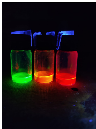
Figure 1: Green-Red Perovskite Nanocrystals under UV Illumination
