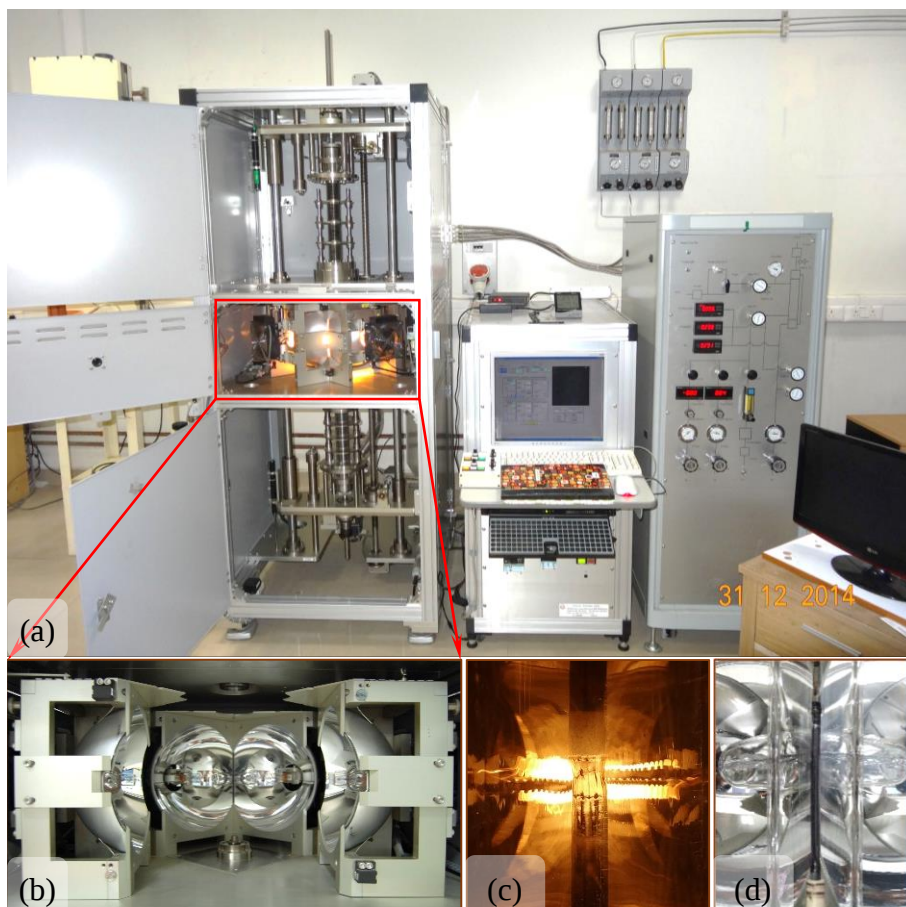
Figure 2.1: (a) Four mirror optical furnace used in the growth experiments (IISER Pune). (b) Close-up image of the four mirrors is shown. (c) Photograph of the dynamical growth process showing feed, molten zone and seed crystal. (d) After the growth process of 5 % Co-doped \text{Sr}_{14}\text{Cu}_{24}\text{O}_{41} crystal is shown inside the furnace.
