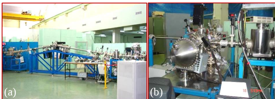
Figure 2.12: (a) The photograph of UGC-DAE-CSR photoelectron spectroscopy beamline (b) Experimental station of angle integrated photoelectron spectroscopy (AIPES) beamline, Indus, RRCAT, Indore, India.
