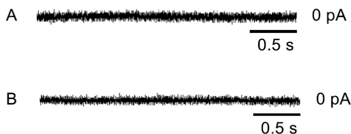
Figure 4.44 Current traces at the applied voltage of 200 mV under symmetrical KCl (1.0 M) conditions across the diphytanoylphosphatidylcholine (diPhyPC) bilayer membrane before (A) and after (B) addition of 1c (20 μM).
