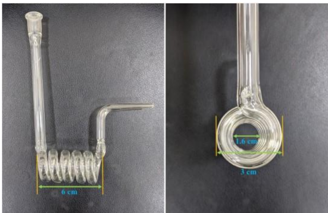
Appendix Scheme 2.5: Digital photograph of continuous flow reactor
