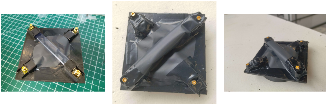
Figure 13: Covered SciCross to filter light from the ambient environment out [(half) LEFT ; (final) MIDDLE & RIGHT].
