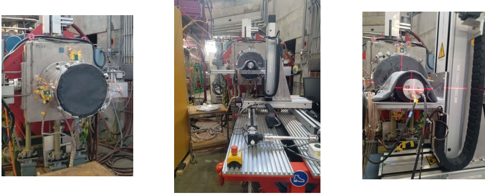
Figure 16: SciFi setup with Tedlar layer for vacuum protection [LEFT] ; Final setup with SciCross-LaBr mounted on the XYZ table [MIDDLE] ; LaBr aligned with the beam on XYZ table [RIGHT].
