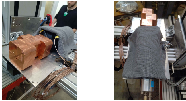
Figure 8: Copper Collimators used during the beamtime. Each of the 3 collimators are 5cm thick and have 4 interchangeable collimation holes of radii 4mm, 3mm, 2mm and 1mm.
