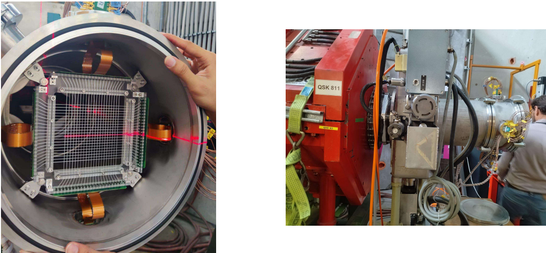
Figure 11: Scintillating Fiber (SciFi) detector horizontally laser aligned with the beam [LEFT] ; Position of SciFi after QSK811 magnet with 855mm of drift space [RIGHT].
