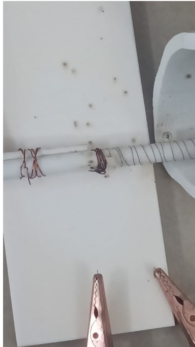
Figure 3.6: Fourth attempt : heater wires at one end got burnt due to excessive voltage applied
