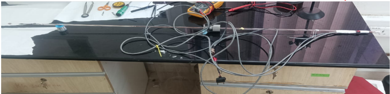
Figure 4.5: Sample Rod 3 : A ceramic rod is inserted in our glass tube as base with heater, sensor and sample mounted on the ceramic rod
