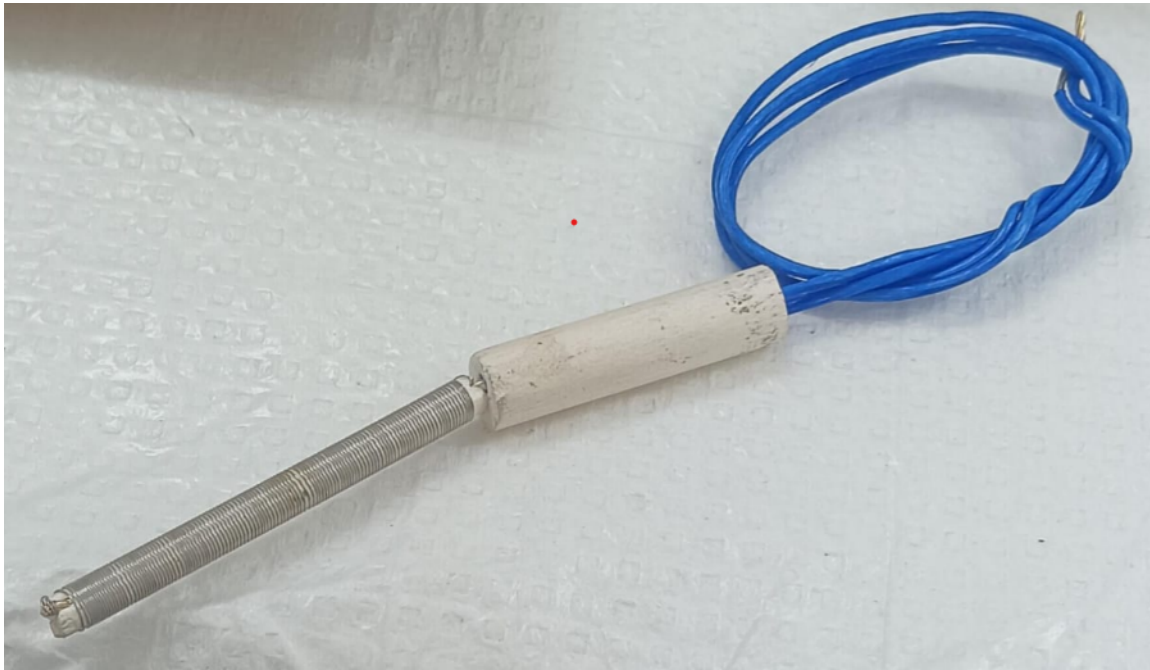
Figure 3.11: Commercial heater used in final run : Nichrome wire wound on a ceramic tube, inductively, with a resistance of around 70\ \Omega
