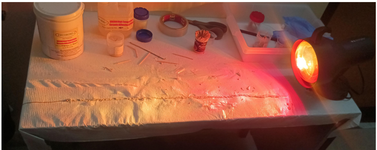
Figure 3.4: Drying cement applied on straight heater wire by using IR lamp
