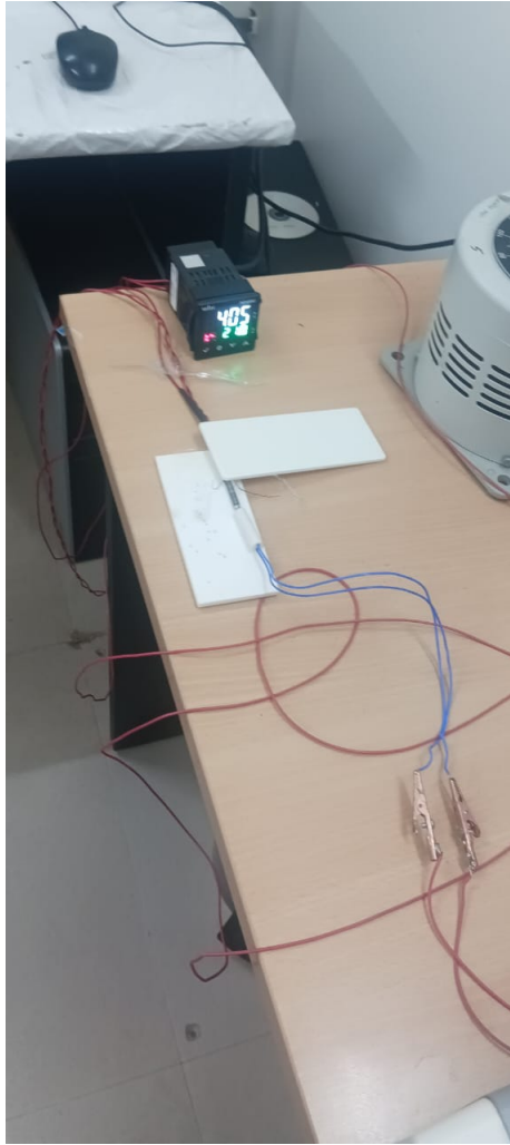
Figure 3.10: Tenth attempt : Heater being tested with PID temperature controller and a dimmerstat without the inconel 800 casing this time
