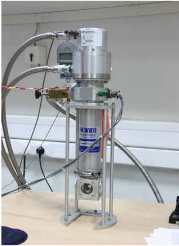
Below: Closed-cycle Refrigerator: Temperatures as low as 4 °K can be reached for studying the temperature dependence of various physical properties.
