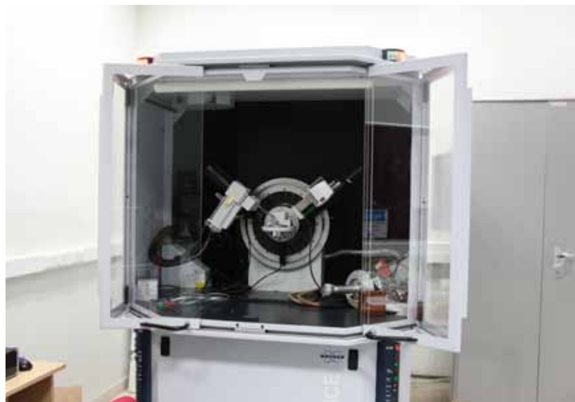
Powder X-ray Diffractometer from Bruker, USA. The diffractometer is equipped with a powerful LYNXEYE detector. It is used to check the phase purity of samples and for carrying out crystal structure refinements.
