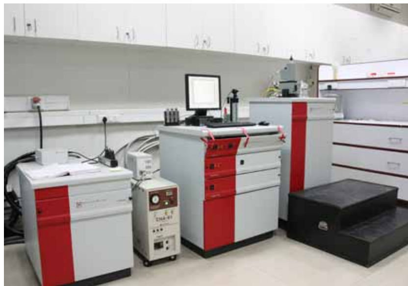
Magnetic Properties Measurement System (MPMS) from Quantum Design, USA. The magnetometer uses a highly sensitive Superconducting Quantum Interference Device (SQUID) for magnetization measurements over wide temperature and magnetic field ranges.
