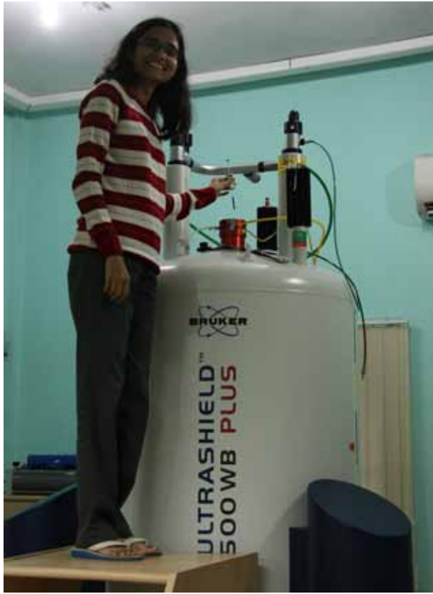
Below: Nuclear Magnetic Resonance (NMR) spectrometer: This 500 MHz Bruker NMR spectrometer operates at a magnetic field of 11.7 Tesla and is capable of controlling nuclear spin dynamics in both liquid and solid state samples. It is being routinely used for quantum information studies as well as for chemical characterization. IISER Pune also has a Bruker 600 MHz, a Bruker 400 MHz, and a JEOL 400 MHz spectrometer.
