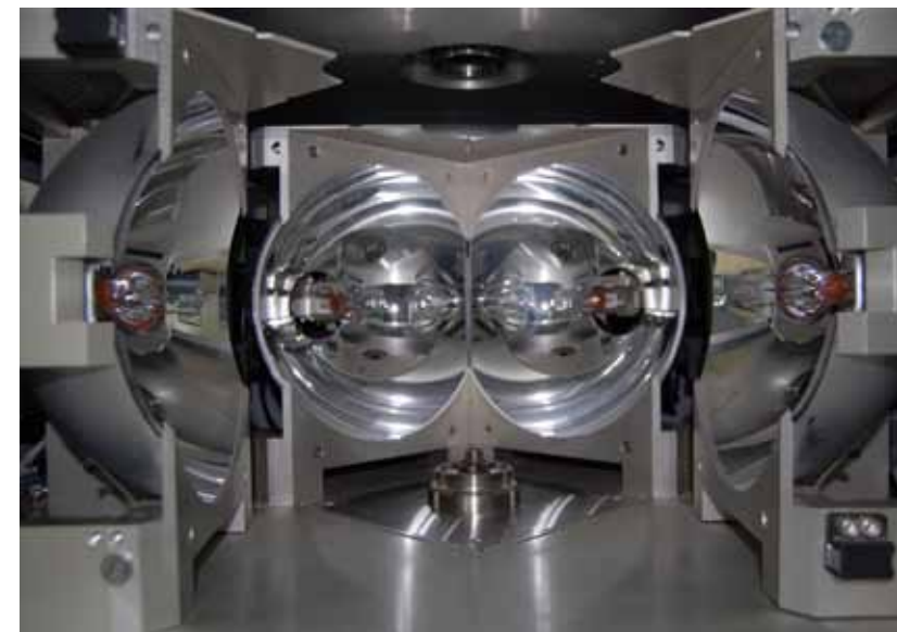
The mirror section of the four-mirror image furnace for single crystal growth. The highly reflecting surfaces are semi-ellipsoidal shaped mirrors. The light flux from halogen lamps is concentrated at their common focal point where temperatures as high as 2500 °C can be reached, sufficient to melt most refractory materials.
