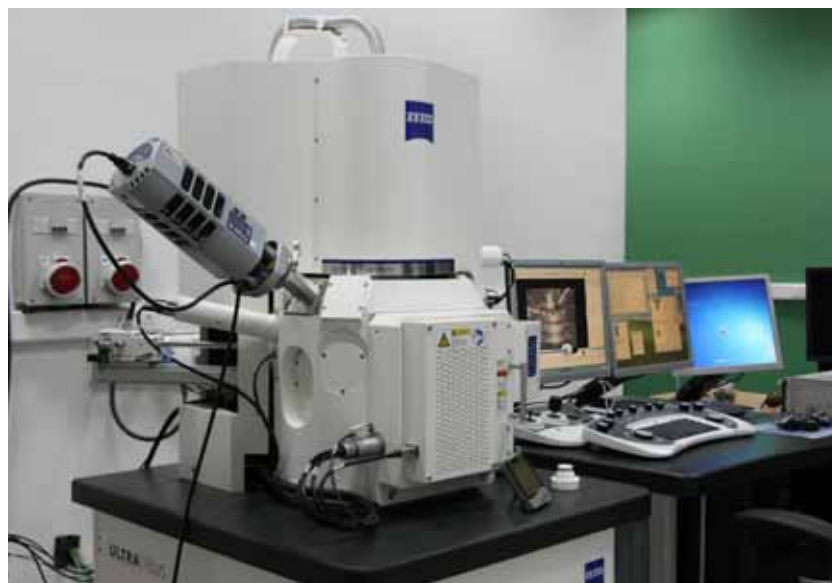
Scanning Electron Microscope from Carl Zeiss. The microscope provides high-resolution images of surfaces and nano-structures. It is equipped with an energy dispersive x-ray analysis tool for composition determination. The system also has an integrated state-of-the-art nano-lithography attachment for device fabrication.
