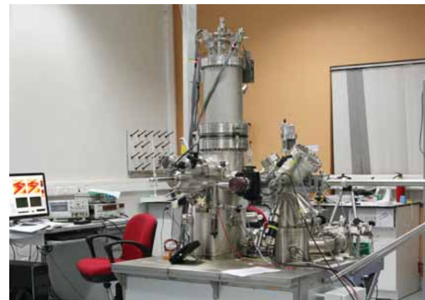
Scanning Tunneling Microscope (STM) from Omicron Germany. Operates in ultra high vacuum (UHV) and at low temperatures for dedicated STM, spectroscopy and atom/molecule manipulation experiments at 77 K and 4.2 K
