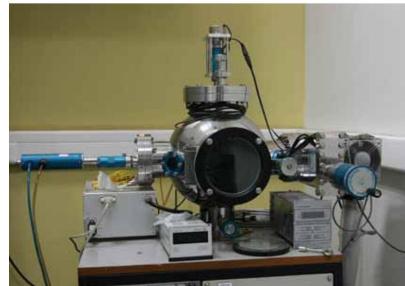
Thin-film Deposition system from Excel Instruments, Mumbai using thermal evaporation technique.
