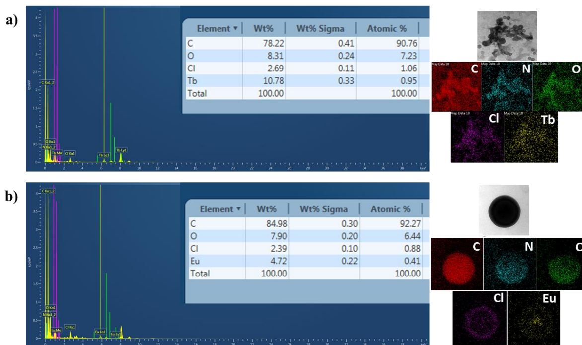
Figure 6: a) EDAX and elemental analysis of P1-TbCl 3 complex. b) EDAX and elemental analysis of P1-EuCl 3 complex.
