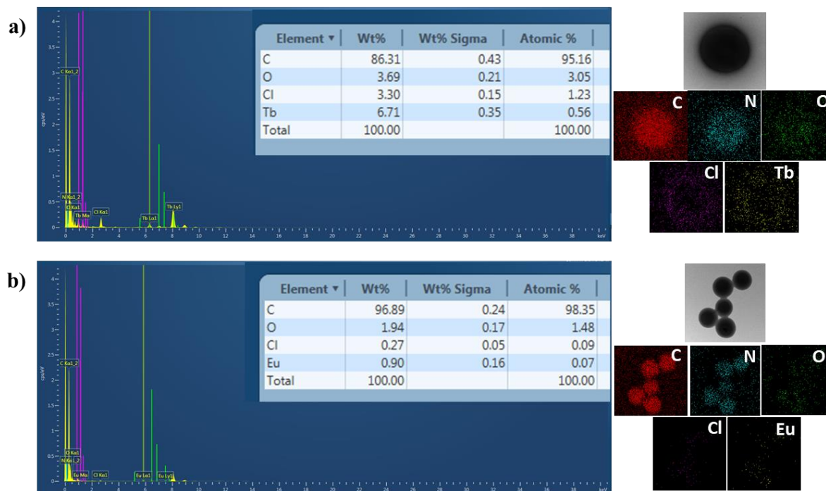
Figure 10: a) EDAX and elemental analysis of P3 -TbCl 3 complex. b) EDAX and elemental analysis of P3 -EuCl 3 complex.
