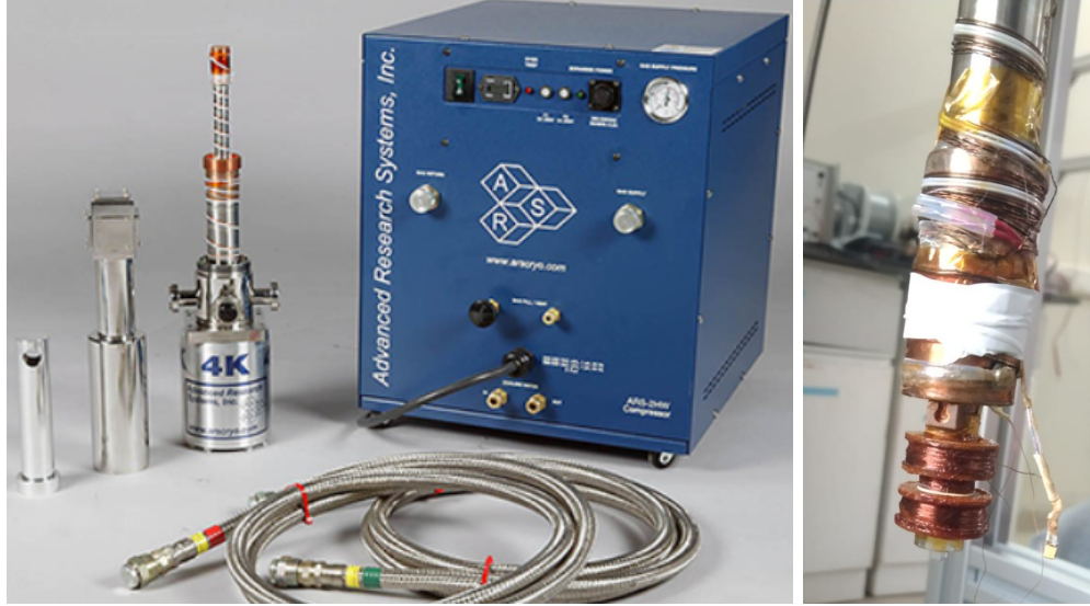
Figure 2.2: 1. A closed-cycle cryostat that has a radiation shield, vacuum shroud, cold head, compressor, and hoses. 2. Sapphire base ac coil attached to the cold finger of the CCR
