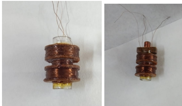
Figure 4.4: 1. Secondary pickup coil winding, 2. Sapphire base AC coil system with copper block sample holder
