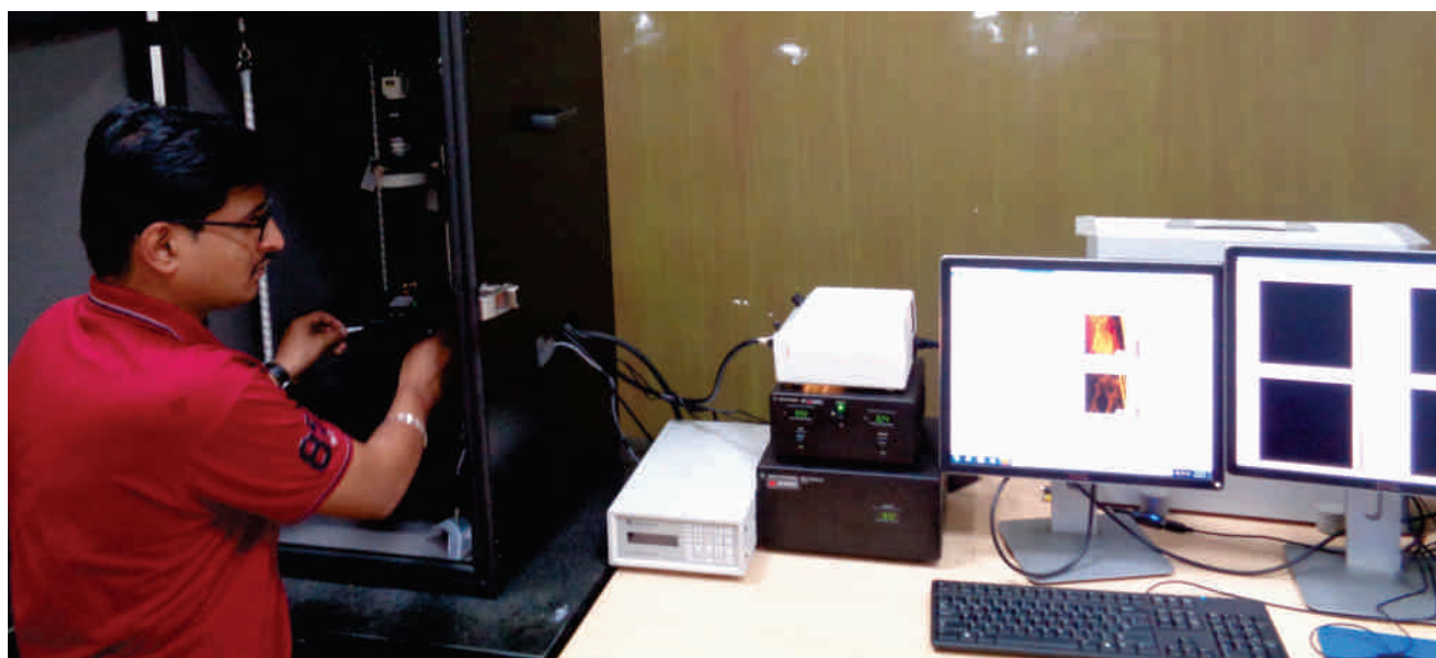
Neelesh Deshpande (PhD student) is seen here with Atomic Force Microscope (5500 Series) for multidisciplinary imaging applications purchased from Keysight Technologies, Singapore Sales Private Ltd, Singapore.
