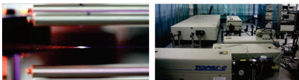
Figure 26: Photographs of THz generating air-plasma (Left) and the experimental set-up (Right) (Dr. Pankaj Mandal's Group)
