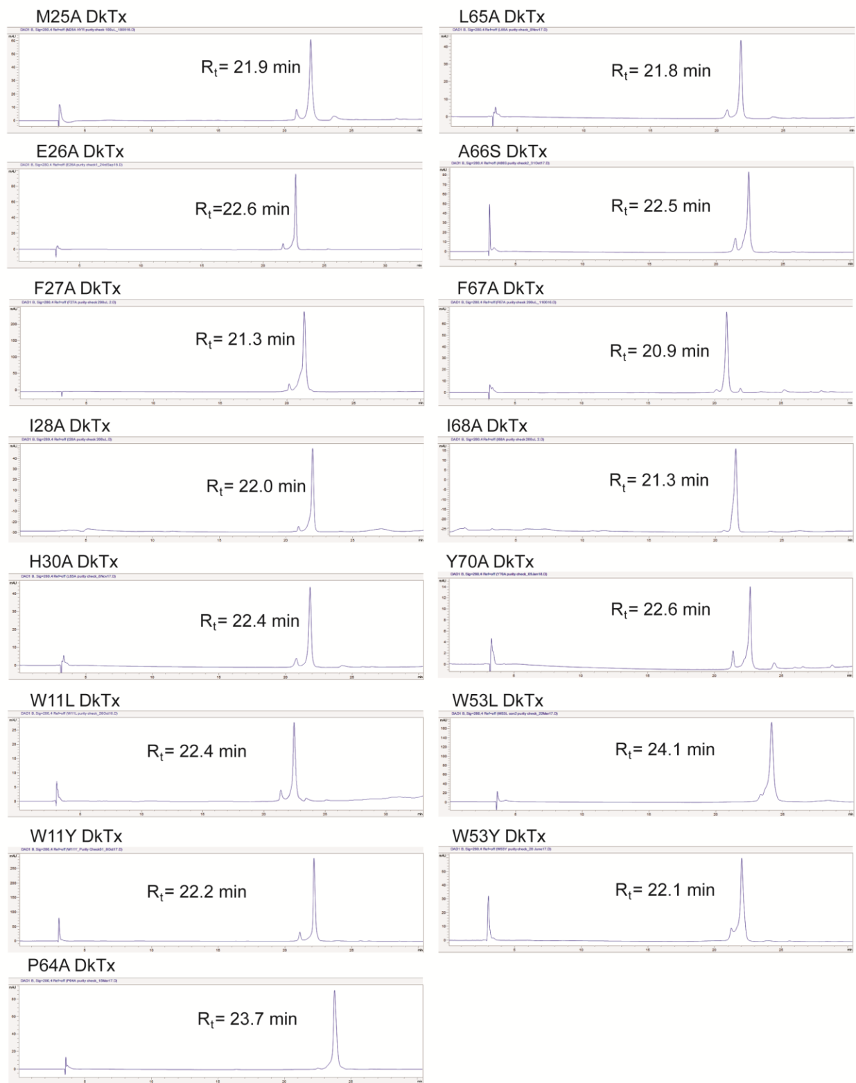
Figure 2.3. HPLC traces for purity evaluation of all our DkTx variants. The absorbance has been measured at 280 nm.
