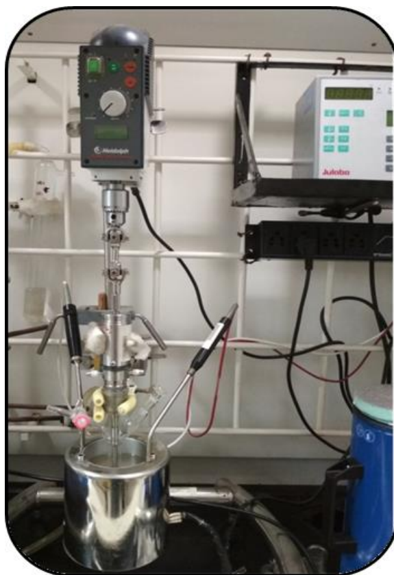
Figure 3.5. Representative image of the in-house specially designed melt reactor set-up with an overhead stirrer and thermocouple
