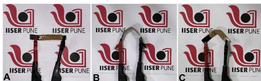
Figure A.3.19. Optical images of the flexible Zn ion battery under different flexible angles.
