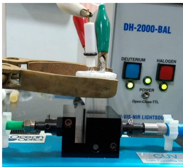
Figure A.2.28. The typical set-up of insitu spectroelectrochemistry.
