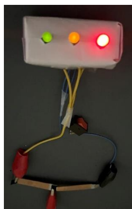
Figure A.3.20. The images show that our flexible Zn ion batteries are able to power 3LEDs (traffic LEDs).
