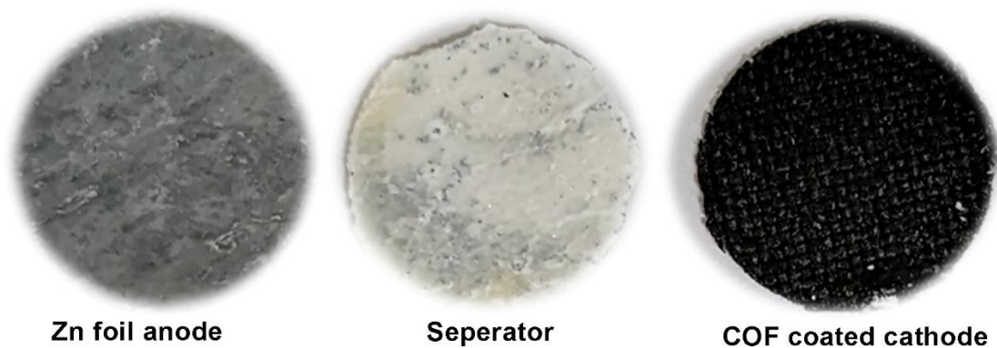
Figure A.3.13. The images show the condition of the anode, cathode, and separator of our of Zn//COF coin cell, fabricated using 3M \text{ZnSO}_4 + 0.2M \text{ZnI}_2 as an electrolyte after 6000 cycles of charge-discharge measurements.
