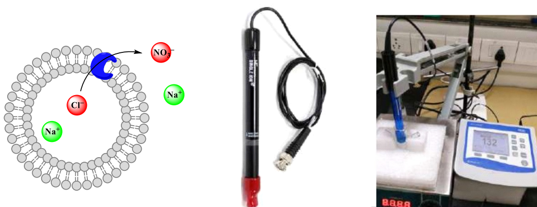
Figure 1.16. Schematic representation of chloride based ion-selective electrode (ISE) and its complete setup.
