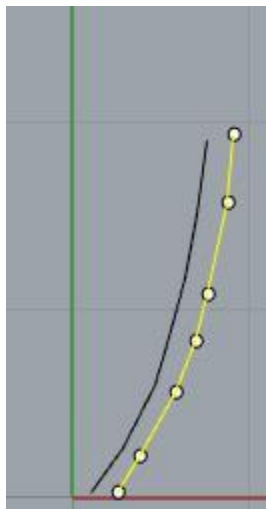
Fig. 16d. Fit between curves in the sub-figure b and the sub-figure c, black curve is natural lineation, and yellow curve is a model curve.
