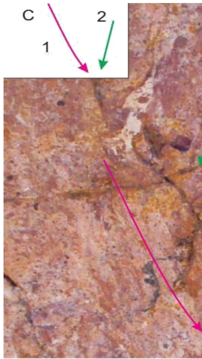
Fig.10a. Natural lineations on fault planes. (from fig. 4c in Xu et al (2013)).
