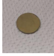
Figure 3.4: Lithium Niobate ( \text{LiNbO}_3 ) disc with Au/Cr coat
