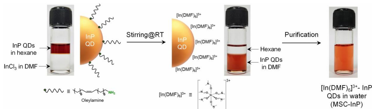
Scheme 5.2. Schematics showing the ligand exchange with positively charged [\text{In}(\text{DMF})_6]^{3+} complex on core-only InP QDs.
