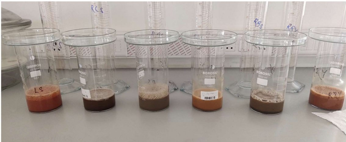
Figure 2.7 Samples after being treated with hydrogen peroxide during the sand-silt-clay separation experiment.
