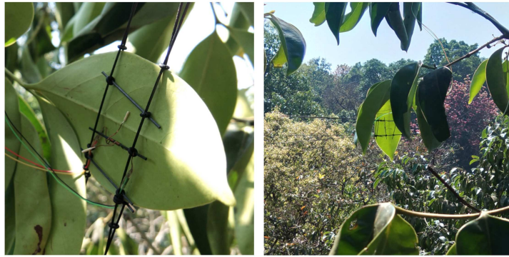
Figure 3.3: Placement of thermistors on the leaves. Left side image shows the underside of a Canthium dicoccum leaf with one thermistor touching the leaf surface and the other to measure the air temperature. The right side picture shows the same leaf in its position in the canopy with the thermistors.
