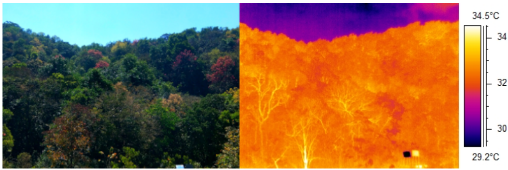
Figure 3.2: RGB and Thermal images of the canopy. The right hand-side picture was taken on the thermal camera on 2023-03-14 12:07:22 IST. The left shows an RGB image of the same canopy. The panels, high emissivity and high reflectivity, used for calibration, can be seen at the bottom right of either images.
