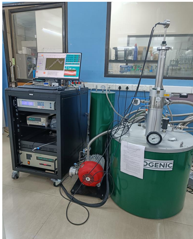
Fig 2.6 CFMS facility for Magneto-transport measurement
