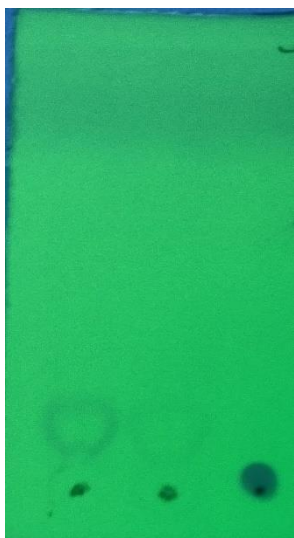
Figure 6.1 TLC of chemoreduction of 7a . First spot – 7a (100 \mu M) control, Second spot – 7a (100 \mu M) + Zn dust (150 mg) + AF (300 \mu M), Third spot – Compound 9. TLC run in 50 % EA:PE
