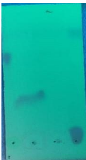
Figure 6.2 TLC of chemoreduction of 7b . First spot – Authentic 7b, Second spot – 7b (50 \mu M) control, Third spot – 7b (50 \mu M) + Zn dust (150 mg) + AF (150 \mu M), Third spot – Compound 9. Left picture – TLC run in 50 % EA:PE twice, Right Picture – TLC run in 50 % EA:PE twice then 70 % EA:PE
